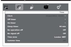
This adjustment allows you to set or to display the following functions: Clock, Off/On Timer and Sleep Timer.
